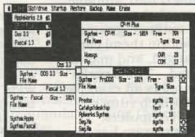
The PlusRAM-16 in this example has been set up using the RamDesk Manager to have four different RAMDisks, one each for AppleWorks (ProDOS), DOS, Pascal and CP/M Plus. The graphics RamDesk Manager shown is for use with the enhanced 128K Apple IIe and Apple IIGS. A text version is also supplied for use with other Apple Models.
